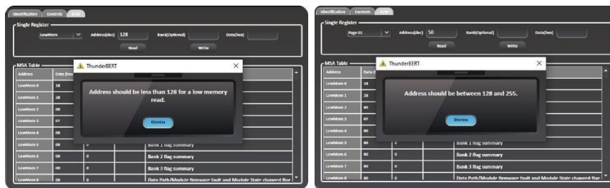
Figure 59: Warning pop-up messages when the address access conditions were not adhered to
